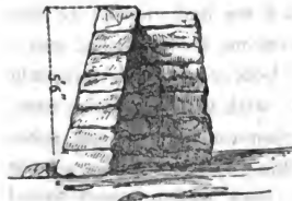
Vertical Section, 5 feet 6 inches high.
